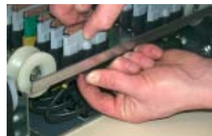
Replacing the carbon brushes.
